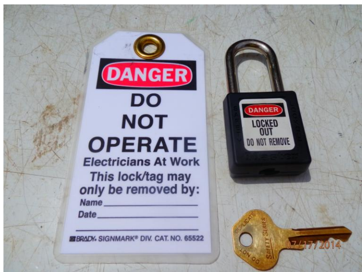
Electricians DANGER TAG and Individual Lock and key
